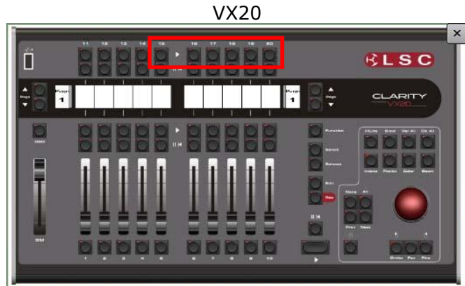
The external inputs control GO buttons 15 to 20
