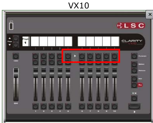
The external inputs control GO buttons 5 to 10
